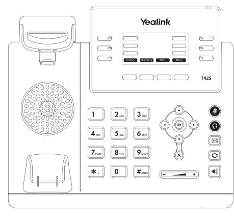
Freely programmable LED keys P1 – P15 Default setting: Line Other settings: Speed Dial, Transfer to, BLF (Busy Lamp Field)
